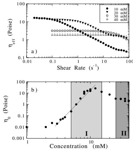
FIG. 3. Rheology of equimolar CPCl/NaSal at 30 °C: (a)  $\eta_{\text{eff}}$  vs  $\dot{\gamma}$  for 10, 20, 30, and 40 mM; (b)  $\eta_0$  as a function of concentration. The shaded regions mark the concentration ranges of bubble oscillations, and the sloped line corresponds to  $\eta_0 \sim \phi^{5.8}$ .
