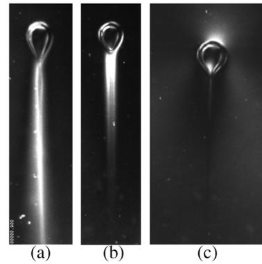
FIG. 4. Birefringent images of the wake behind a bubble rising in CPCl/NaSal at  $T = 24$  °C: (a) 10 mM; (b) 20 mM; (c) 35 mM. Each image is 6.5 cm high. Reynolds and Deborah numbers for each image are (a)  $Re \approx 4.72$ ,  $De \approx 250$ ; (b)  $Re \approx 0.02$ ,  $De \approx 6$ ; (c)  $Re \approx 1.1$ ,  $De \approx 1.8$ .
