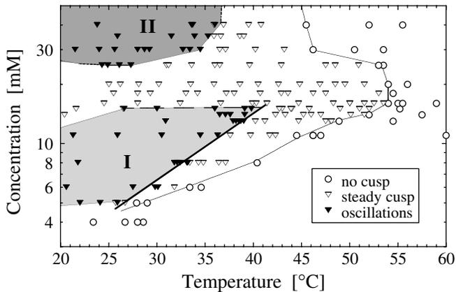
FIG. 2. Temperature and concentration phase diagram for the dynamics of rising bubbles in equimolar CPCl/NaSal, showing two distinct regions of oscillating behavior (shaded) labeled as I and II. The thick sloped line marking the temperature boundary for type I oscillations is an isoline of Eq. (1).
