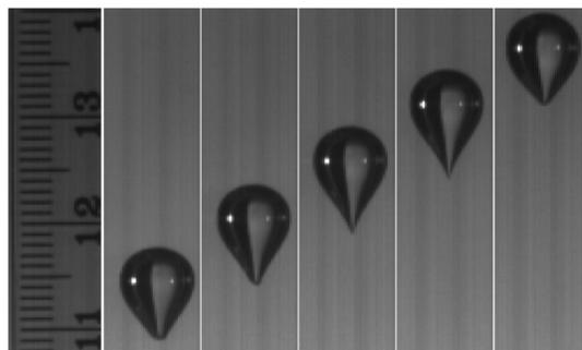
FIG. 1. Cusp shape change of an oscillating bubble rising through a 15 mM CPCl/NaSal (weight fraction  $\varphi = 0.5\%$ ) solution at  $T = 37.5^\circ\text{C}$ . The scale at left is marked in centimeters. Interval between pictures: 0.05 s.
