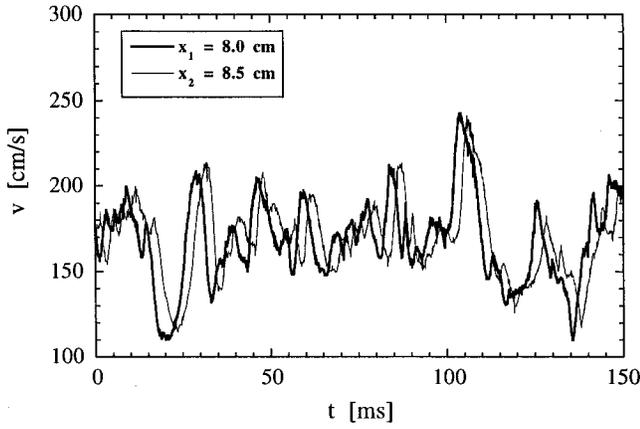
FIG. 3. Simultaneous traces of the velocity versus time at  $x_1 = 8.0$  cm and  $x_2 = 8.5$  cm behind the comb.
