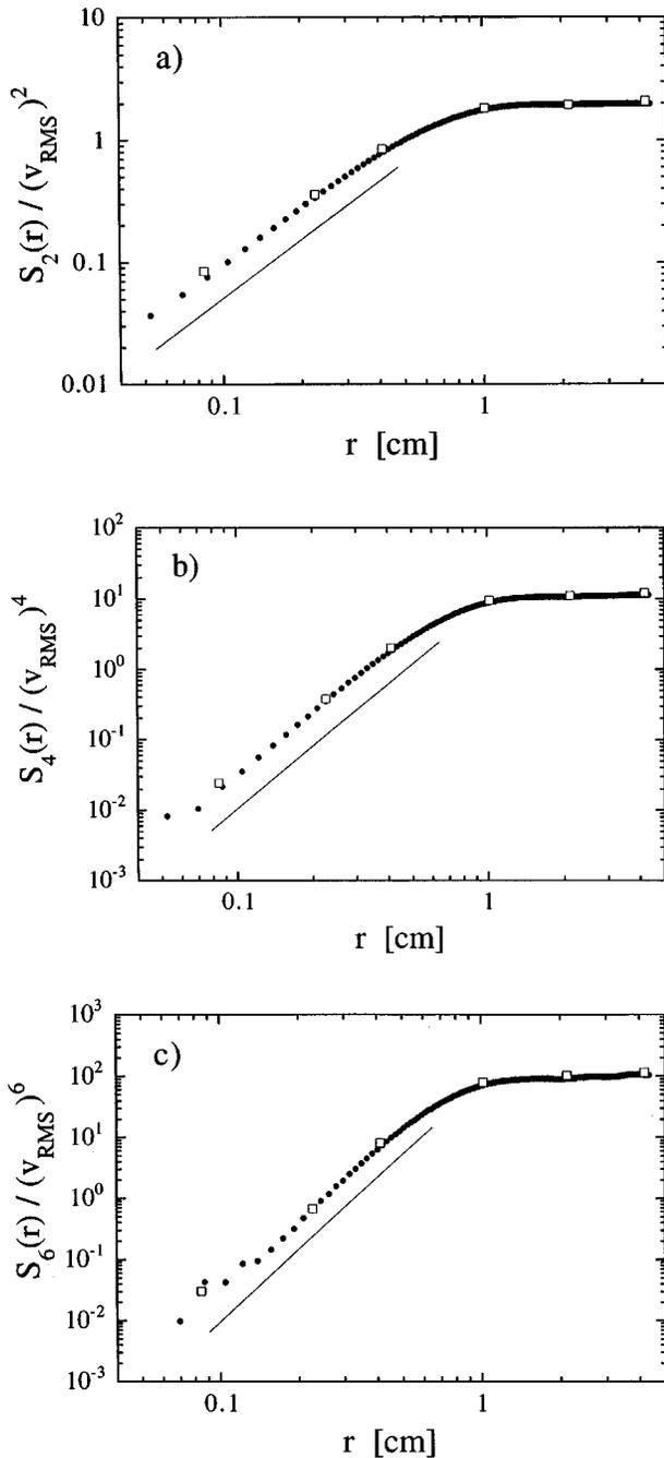
FIG. 7. Experimental check of Taylor's hypothesis for (a) second order structure function  $S_2(r)$  taken at  $x = 8$  cm using Taylor's hypothesis; (b) fourth order structure function  $S_4(r)$ ; (c) sixth order structure function  $S_6(r)$ . The open squares are direct spatial measurements made using two probes, and the lines correspond to the fitted scalings described in the text.
