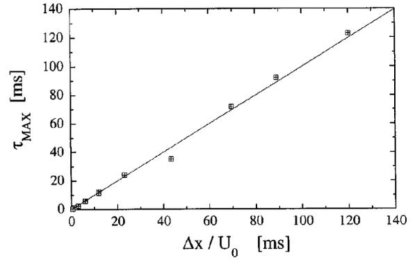
FIG. 5. The delay time  $\tau_{\text{MAX}}$  for the maximum of the cross correlations in Fig. 4 versus the transit time  $\Delta x/U_0$ . The solid line corresponds to  $\tau_{\text{MAX}} = \Delta x/U_0$ .
