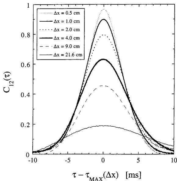
FIG. 18. An overlay of several  $C_{12}(\tau)$  at various  $\Delta x$  (as shown), plotted versus  $\tau - \tau_{\text{MAX}}(\Delta x)$ .
