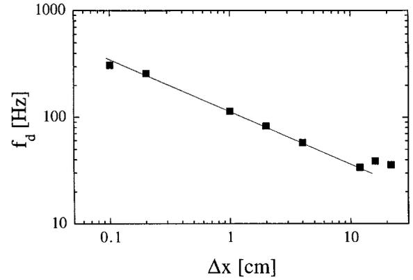
FIG. 13. The frequency scale  $f_d$  of the logarithmic decay  $C_s(f) \sim \log(1/f)$  (lines in Fig. 11) versus  $\Delta x$ . The straight line represents the scaling  $f_d \sim \Delta x^{-1/2}$ .
