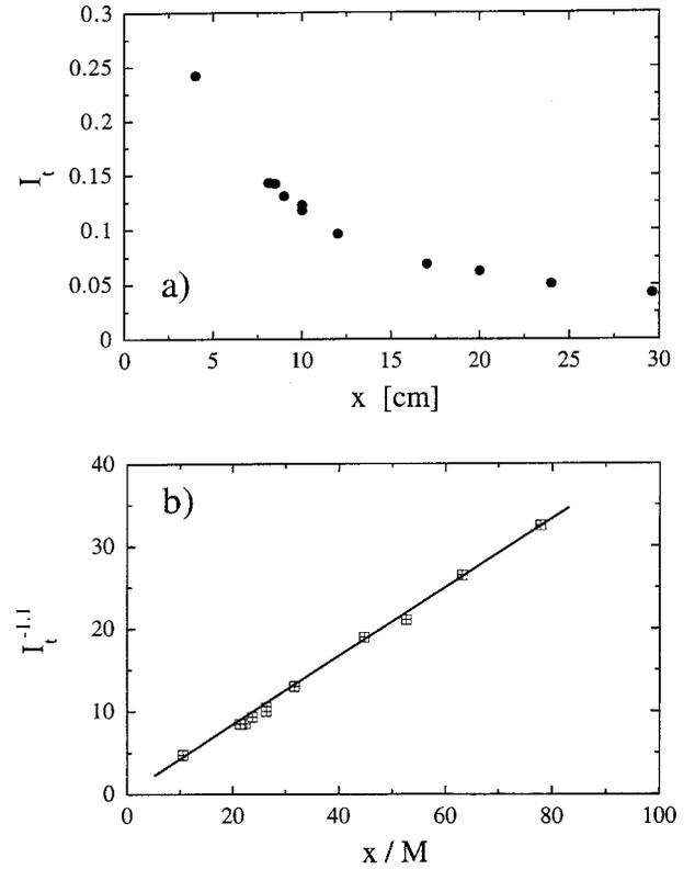
FIG. 2. The decay of the turbulent intensity  $I_t$  behind the comb in our soap film: (a)  $I_t$  versus downstream distance  $x$ ; (b) the same data plotted as  $I_t^{-1.1}$  vs  $x/M$ . The straight line is a linear fit (see the text).
