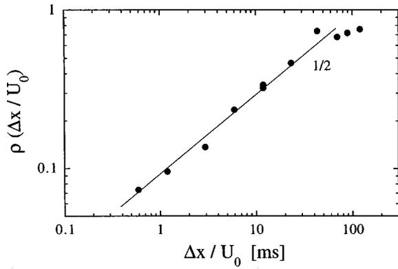
FIG. 15. A log-log plot of  $\rho(\Delta x/U_0)$  as a function of downstream time  $\Delta x/U_0$ . The straight line corresponds to a power law dependence  $(\Delta x/U_0)^{1/2}$  (see the text).
