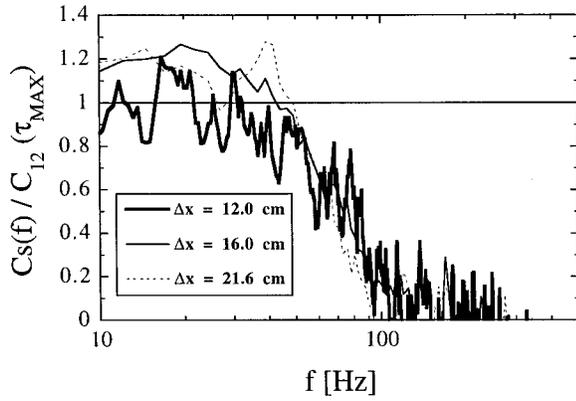
FIG. 12. Coherence spectra for several large values of  $\Delta x$  as a linear-log plot of  $f$ , normalized by the maximum cross correlation  $C_{12}^{\text{MAX}}$  from Fig. 6.
