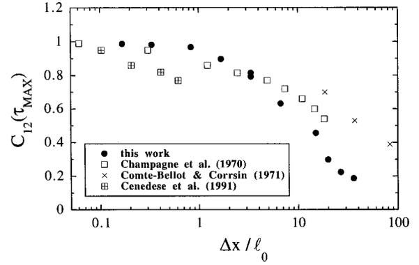
FIG. 16. A replot of  $C_{12}^{\text{MAX}}$  from Fig. 6 as a function of probe separation  $\Delta x$  normalized by the integral scale  $l_0$ . Also shown for comparison are 3-D results from Refs. 21, 22, and 23.
