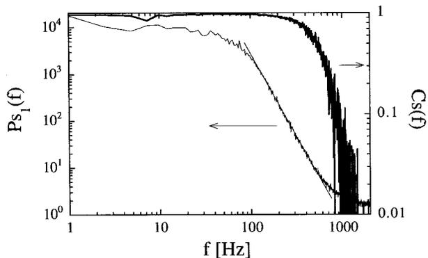
FIG. 9. A comparison of the coherence spectrum [Eq. (3)] for  $\Delta x = 0.2$  cm, and the power spectrum taken at  $x_1 = 8$  cm. The line is a fit to the power law  $Ps_1(f) \sim f^{-\alpha}$  with  $\alpha = 3.6 \pm 0.2$ .
