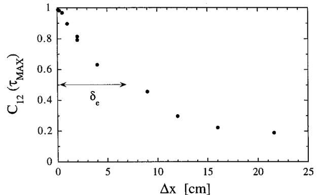
FIG. 6. The maximum value of the cross correlations in Fig. 4,  $C_{12}^{\text{MAX}}$  versus the downstream separation  $\Delta x$ . The arrow shows the evolution length  $\delta_e \approx 7$  cm (see the text).
