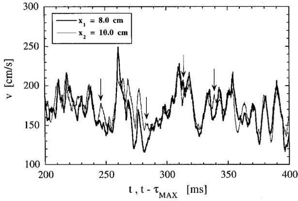
FIG. 8. Overlay of the velocity measured at  $x_1 = 8.0$  cm versus  $t$ , and the velocity measured at  $x_1 = 10.0$  cm versus  $t - \tau_{MAX}$ . The arrows indicate fluctuation spikes which have either appeared or disappeared during the transit between the two probes.
