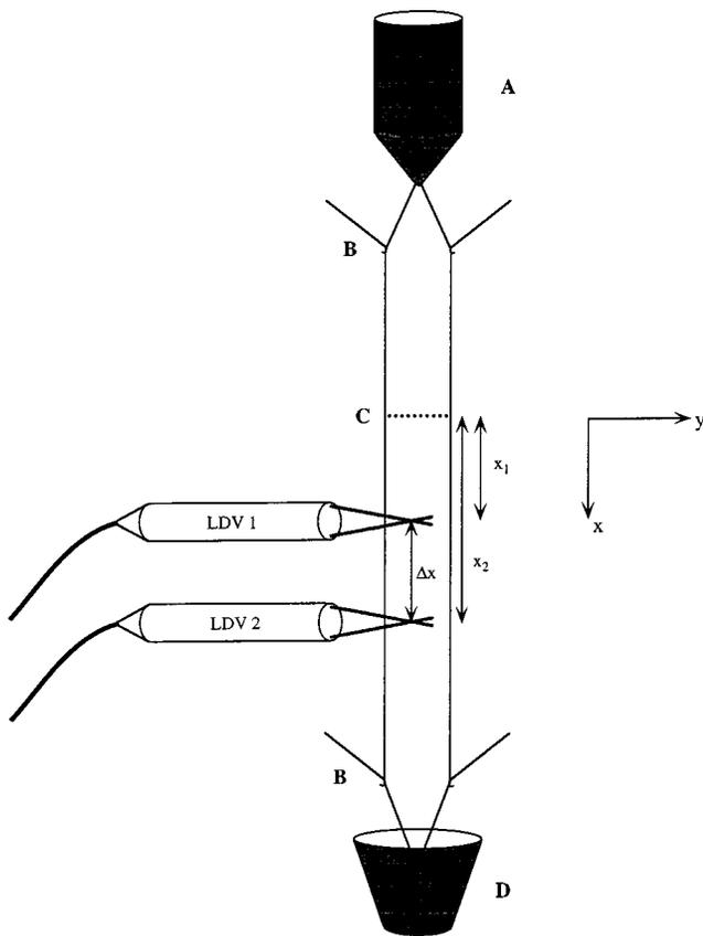
FIG. 1. A diagram of the experimental setup: (a) upper soap reservoir; (b) hooks which hold plastic wires between which soap film flows; (c) comb behind which turbulence is generated in the film; (d) lower soap reservoir. The two LDV probes which measure the velocity in the film are labeled 1 and 2. Downstream distances are labeled as referred to in the text.
