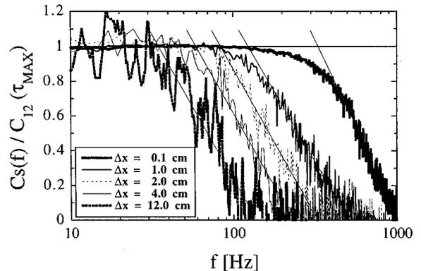
FIG. 11. Coherence spectra as in Fig. 10 normalized by the maximum cross correlation  $C_{12}^{MAX}$  from Fig. 6. The straight lines through the high frequency part of the coherence spectra corresponds to  $Cs(f) \sim \log(1/f)$ .
