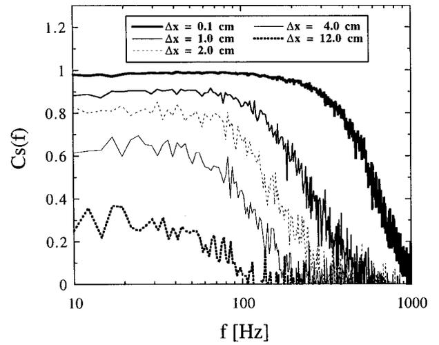
FIG. 10. Coherence spectra for several values of  $\Delta x$  as a linear-log plot of  $f$ .
