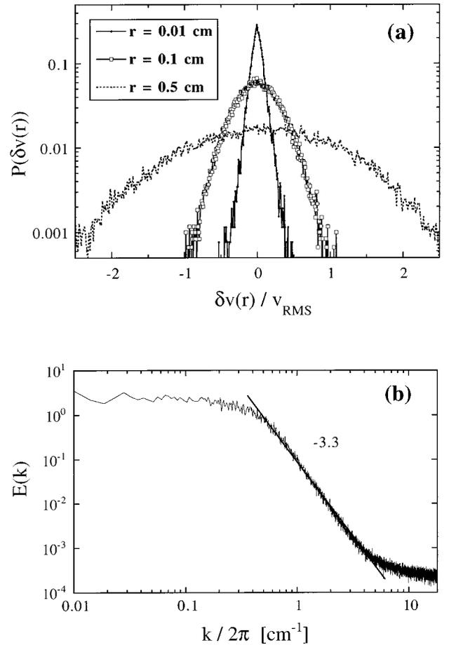
FIG. 2. (a) The PDFs of  $\delta v(r)$  at the three indicated values of  $r$ . (b) Energy spectrum obtained from the time series of the longitudinal velocity, showing an interval where  $E(k) \sim k^{-3.3}$ . The data in both plots are taken at  $Y = 8$  cm.
