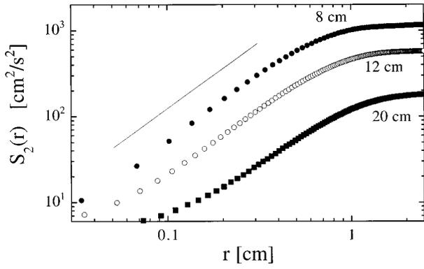
FIG. 3. Log-log plot of  $S_2(r)$  vs.  $r$  at the indicated distances ( $Y$ ) below the comb; the solid line corresponds to  $S_2(r) \propto r^{1.6}$ .
