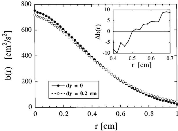
FIG. 5. The velocity correlation function  $b(r)$  measured at two different downstream distances, separated by 0.20 cm, at  $Y=8.6$  cm. The inset shows the difference  $\Delta b$  of these two curves near their crossing point; note that  $\Delta b > 0$  at large  $r$ .
