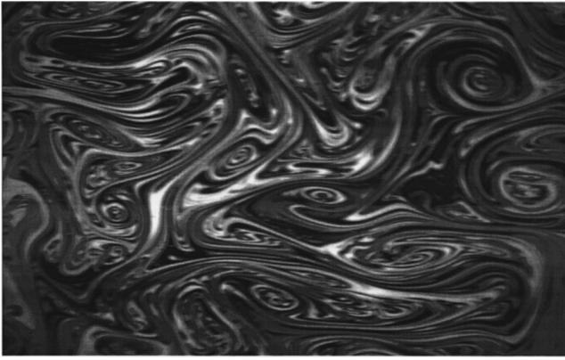
FIG. 1. The central region of the turbulent soap film,  $Y=8$  cm behind comb. The image is about 4 cm across, and the flow is from right to left. The mean flow speed is 180 cm/sec.
