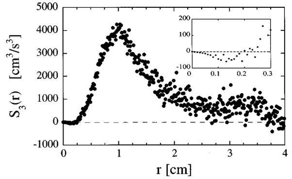
FIG. 4. The third moment  $S_3(r)$  (linear scale) measured at  $Y = 8.0$  cm; the dashed line is  $S_3(r) = 0$ . The inset is an enlargement at small  $r$ .
