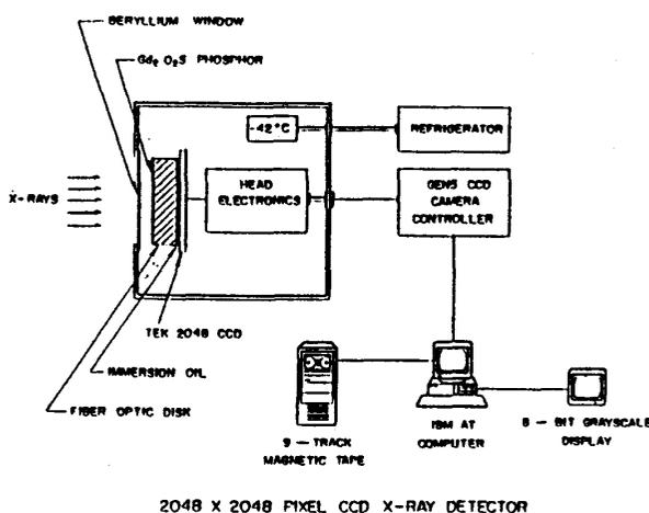
Fig. 1 Schematic diagram of the detector.
