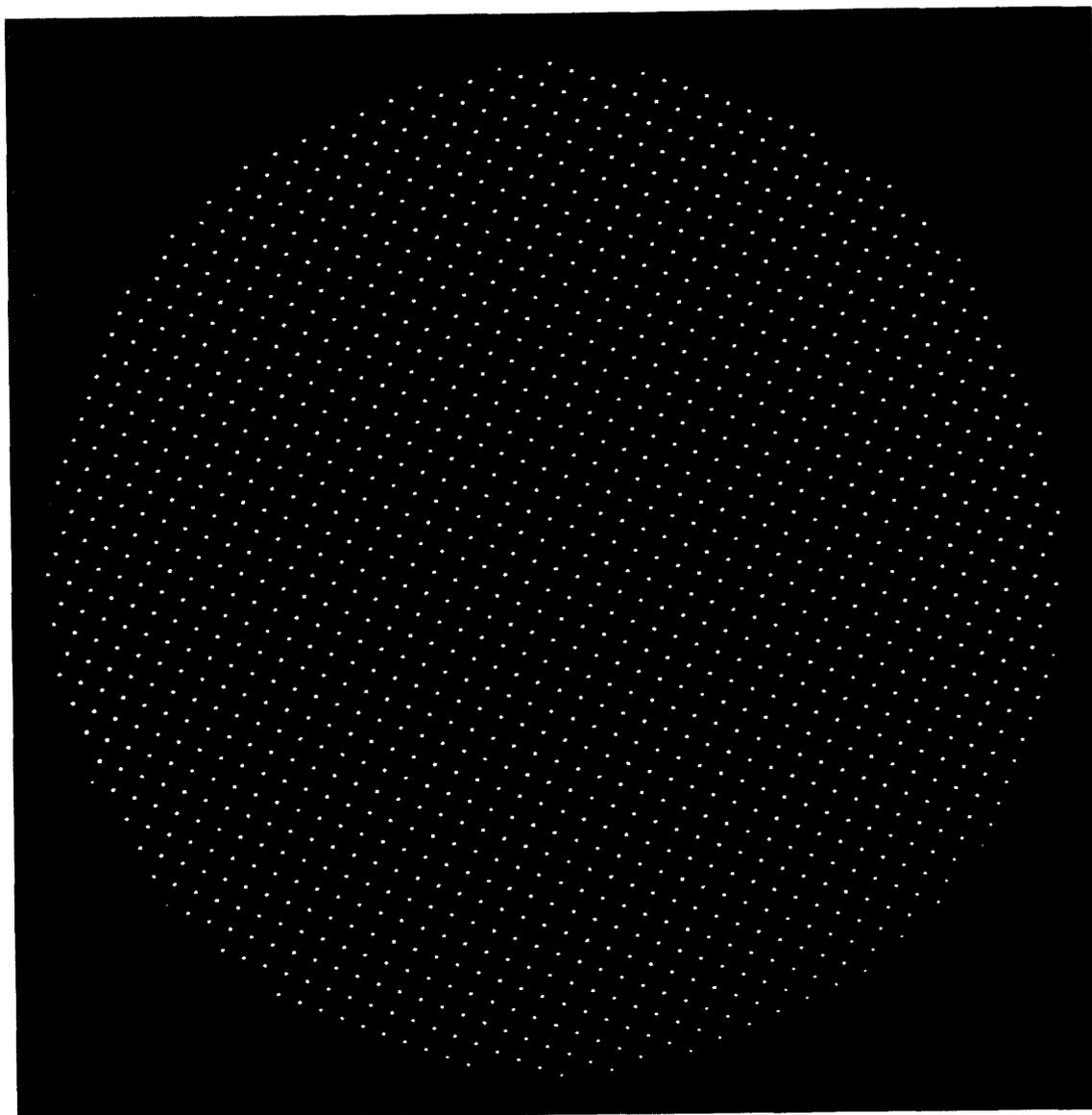
Figure 4 X-ray image of the test mask. The holes in the tungsten sheet are  $75 \mu\text{m}$  in diameter and lie on 1 mm centers.
