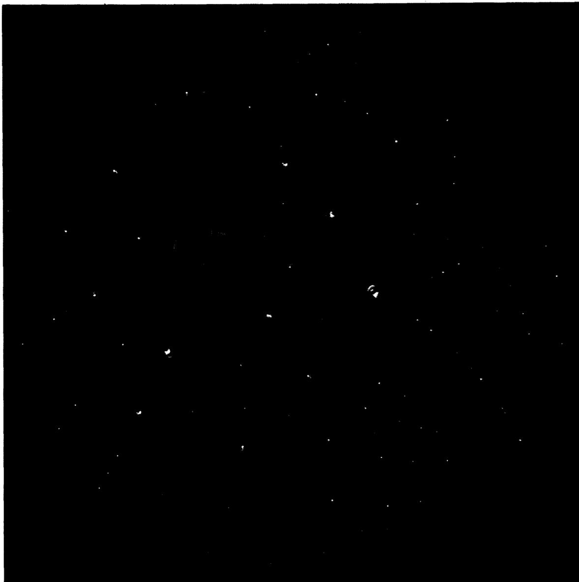
Fig. 8 Laue diffraction pattern of tetragonal lysozyme recorded with an x-ray beam collimated to 20  $\mu\text{m}$  diameter. The exposure time was 2 s, and the beam intensity was estimated to be  $10^{11}$  x-ray/s.
