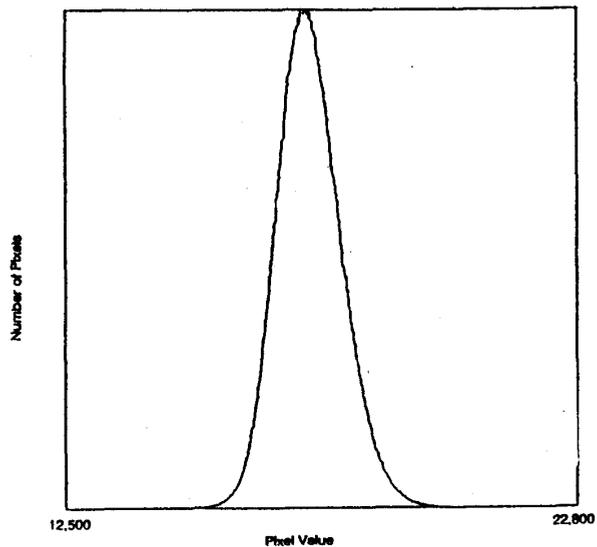
Fig. 3 Histogram of the values of  $10^6$  pixels exposed to uniform illumination by Ni filtered Cu radiation. The mean value corresponds to 11,500 x-ray/pixel, and the FWHM is 8% of the mean.
