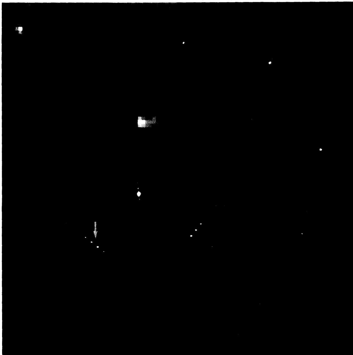
Fig. 5 Laue diffraction pattern of a gallium arsenide/gallium aluminum arsenide multilayered crystal recorded with an x-ray beam collimated to 20  $\mu\text{m}$  diameter. The exposure time was 1 s, and the beam intensity was estimated to be  $10^{11}$  x-ray/s. The inset shows a 32 $\times$  enlargement of the reflections on either side of the arrow.
