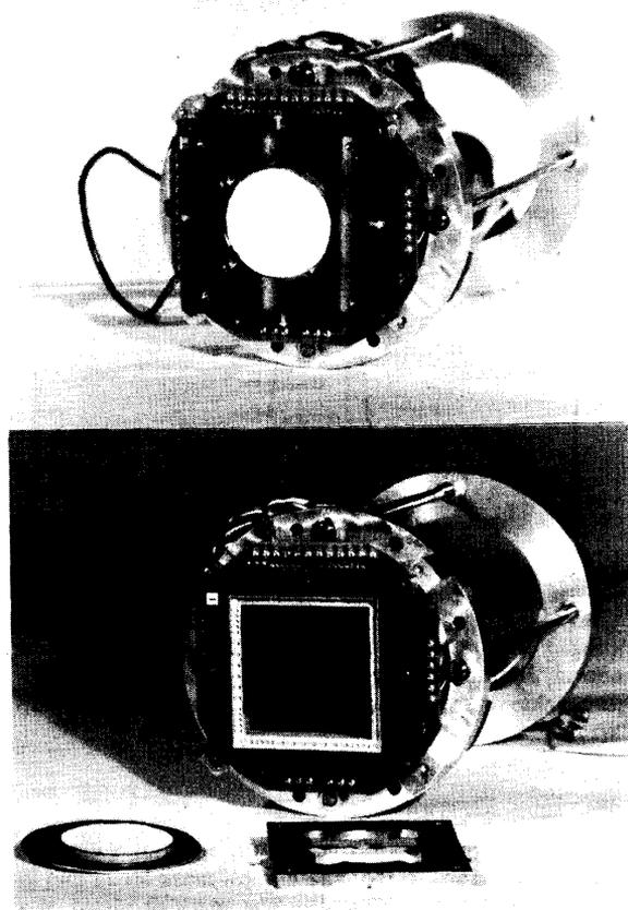
Fig. 2 (Top) Photograph of the CCD carrier with the 50 mm diameter fiber optic disk and phosphor in place. This assembly slides into the cooled copper jacket of the cryostat to position the phosphor 25 mm behind the beryllium window. (Bottom) Photograph of the CCD carrier with the fiber optic disk (lower left) and its brass holder (lower right) removed. The CCD is seen at the center. The silicon die, including the wire bonding pads, measures 85 mm across the diagonal.
