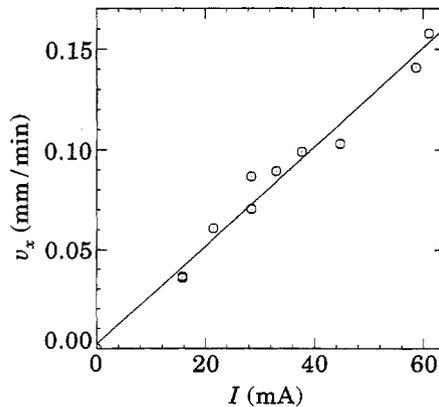
Fig. 4. – The spiral drift velocity parallel to the applied current ( $v_x$ ) in mm/min, as a function of applied current  $I$  in mA.
