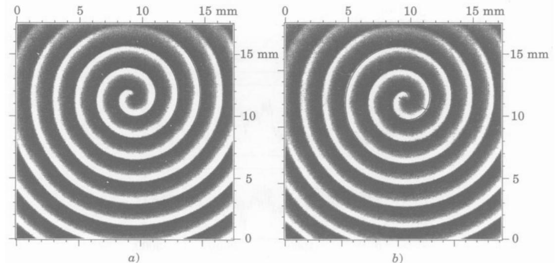
Fig. 2. – a) A free spiral ( $I = 0$ ), with the best Archimedean fit superimposed. The cross marks the centre of the fitted spiral ( $\alpha = 0.014$ ). b) A spiral with  $I = 37.8$  mA (the anode is on the right), with the trajectory of the centre superimposed ( $x_c$  vs.  $y_c$ ). The image shown is at  $t = 700$  s, at the spiral's maximum distortion ( $\alpha = 0.04$ ).
