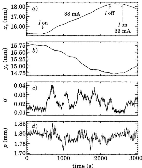
Fig. 3. - The drift and distortion of the spiral vs. time: a)  $x_c$ , b)  $y_c$ , c) distortion parameter  $\alpha$ , d) pitch  $p$ . From  $t = 420 \text{ s}$  to  $t = 2220 \text{ s}$ ,  $I = 37.8 \text{ mA}$ . From  $t = 2580 \text{ s}$ ,  $I = -33.1 \text{ mA}$ . Note the difference in scale between  $x$  and  $y$ . The rapid oscillations in  $p$  at the rotation frequency are an artifact of the analysing method.
