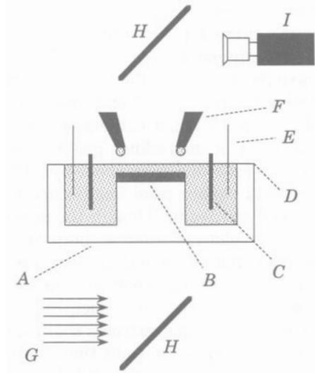
Fig. 1. – A diagram of the experimental apparatus: A: plexiglas cell (7 cm long); B: gel; C: glass baffles; D: evacuation point for solution; E: electrodes; F: nozzles for fresh solution; G: parallel illumination; H: mirrors; I: camera. The reaction only takes place in the gel, where the ferroin is confined; the solution filling the cell is represented in dotted grey.
