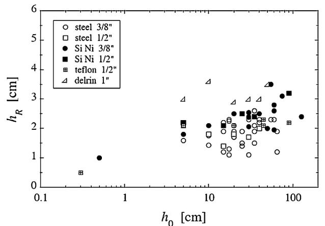
Fig. 6. The rebound height  $h_R$  as a function of the initial drop height  $h_0$ , for different spheres in our experiments.
