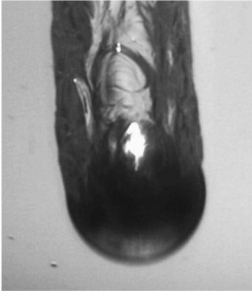
Fig. 12. Closeup of the surface where the micellar fluid meets a falling  $d = 0.95$  cm steel sphere, in a different experiment than Figs. 10 and 11. The sphere was dropped from  $h_0 = 70$  cm, and at the depth shown (about 6 cm below the surface) has an estimated speed of 200 cm/s ( $Re \simeq 0.44$ ,  $De \simeq 420$ ).
