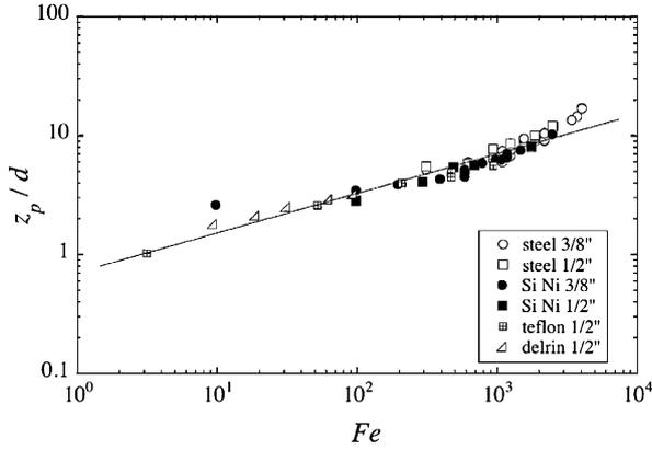
Fig. 4. Non-dimensional plot of the penetration depth  $z_p/d$  vs. the elastic Froude number  $Fe$  (see text) for six different data sets. The straight line corresponds to the scaling law  $z_p/d \sim Fe^{1/3}$ .
