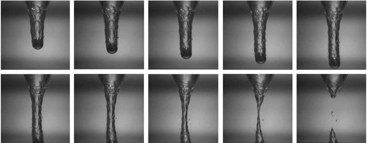
Fig. 10. Cavity dynamics for a  $d = 0.95$  cm steel sphere dropped from  $h_0 = 70$  cm, shown every 2.0 ms ( $Re \simeq 0.82$ ,  $De \simeq 780$ ;  $Fe \simeq 4 \times 10^3$ ).
