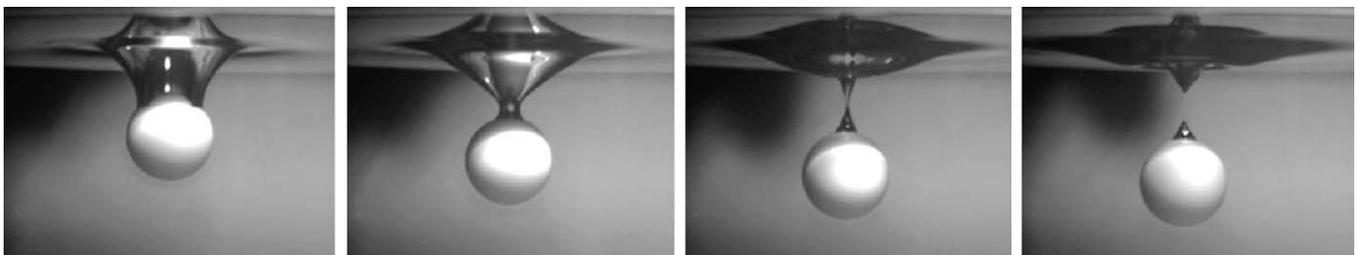
Fig. 7. Cavity formation for a  $d = 2.54$  cm delrin sphere dropped from  $h_0 = 5$  cm ( $Re \simeq 0.58$ ,  $De \simeq 78$ ;  $Fe \simeq 16$ ), characteristic of the ‘smooth’ cavity surface state. The images shown are separated by 20 ms.
