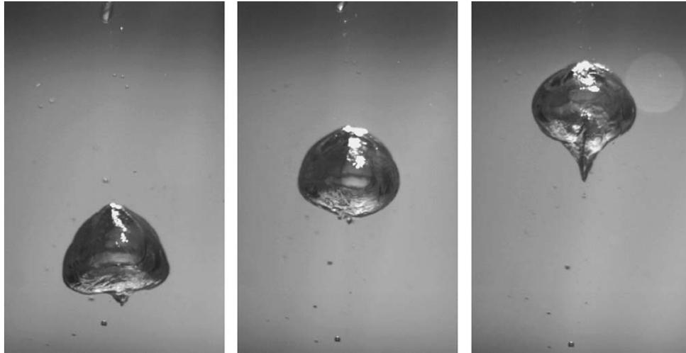
Fig. 15. After the impact of a  $d = 1.27$  cm steel sphere falling from  $h_0 = 70$  cm, a large air bubble (about  $2\text{ cm}^3$ ) entrained by the sphere rises through the fluid. The images are separated by  $\Delta t = 33$  ms.
