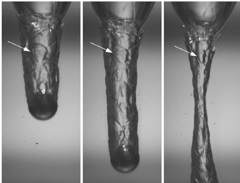
Fig. 11. Closeup of the development of surface texture in the cavity behind a  $d = 0.95$  cm steel sphere dropped from  $h_0 = 70$  cm ( $Fe \simeq 4 \times 10^3$ ). The arrow indicates a scallop-shaped fracture which remains at the same depth while the sphere plunges downwards (frames shown are separated by 8 ms).
