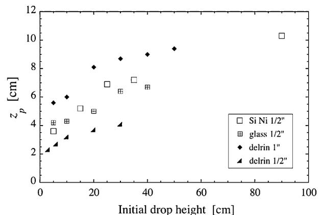
Fig. 3. Dependence of the penetration depth  $z_p$  on the initial drop height  $h_0$  for several different spheres in our experiment.
