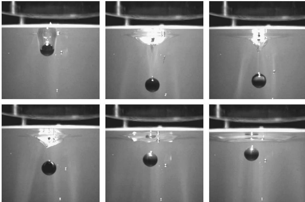
Fig. 1. Sequential images of the penetration of a 0.95 cm diameter silicone nitride sphere dropped from  $h_0 = 30$  cm into 80/60 mM CPCI/NaSal solution ( $Re \simeq 0.5$ ,  $Fr \simeq 60$ ,  $Fe \simeq 590$ ). The time between images is 40 ms.
