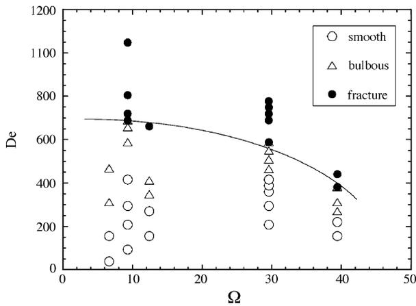
Fig. 13. Texture of the cavity surface for the experiments, shown as a function of Deborah number  $De$  and elastic Grashof number  $\Omega$  (Eq. (2)).
