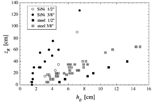
Fig. 5. Dependence of the position of the first rebound  $z_R$  on the initial drop height  $h_0$  for several different spheres in our experiment.
