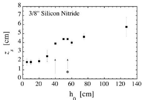
Fig. 14. Cavity seal depth  $z_s$  as a function of drop height  $h_0$  for (a)  $d = 0.95$  cm steel sphere; (b)  $d = 0.95$  cm silicon nitride sphere. The error bars show the range of variation of the data.
