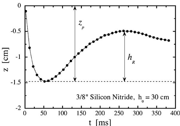
Fig. 2. The dynamics after impact (depth  $z$  vs. time) of a silicon nitride sphere,  $d = 0.95$  cm,  $h_0 = 30$  cm (same experiment as Fig. 1).
