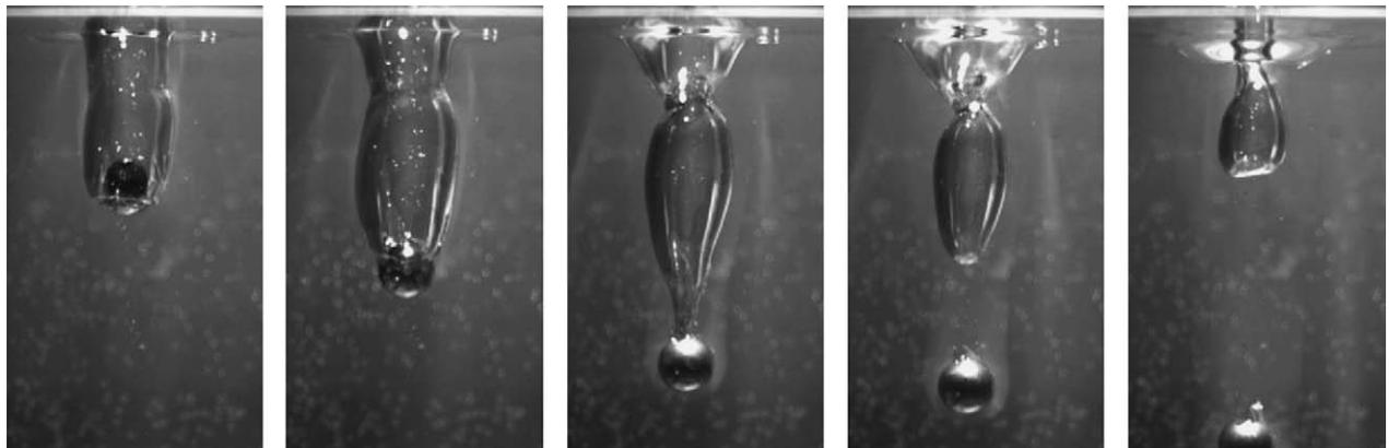
Fig. 9. Cavity dynamics for a  $d = 0.95$  cm steel sphere,  $h_0 = 30$  cm ( $Re \simeq 0.53$ ,  $De \simeq 510$ ;  $Fe \simeq 1860$ ), shown after the moment of impact at  $t$  (a) 13 ms; (b) 21 ms; (c) 33 ms; (d) 37 ms; (e) 53 ms.
