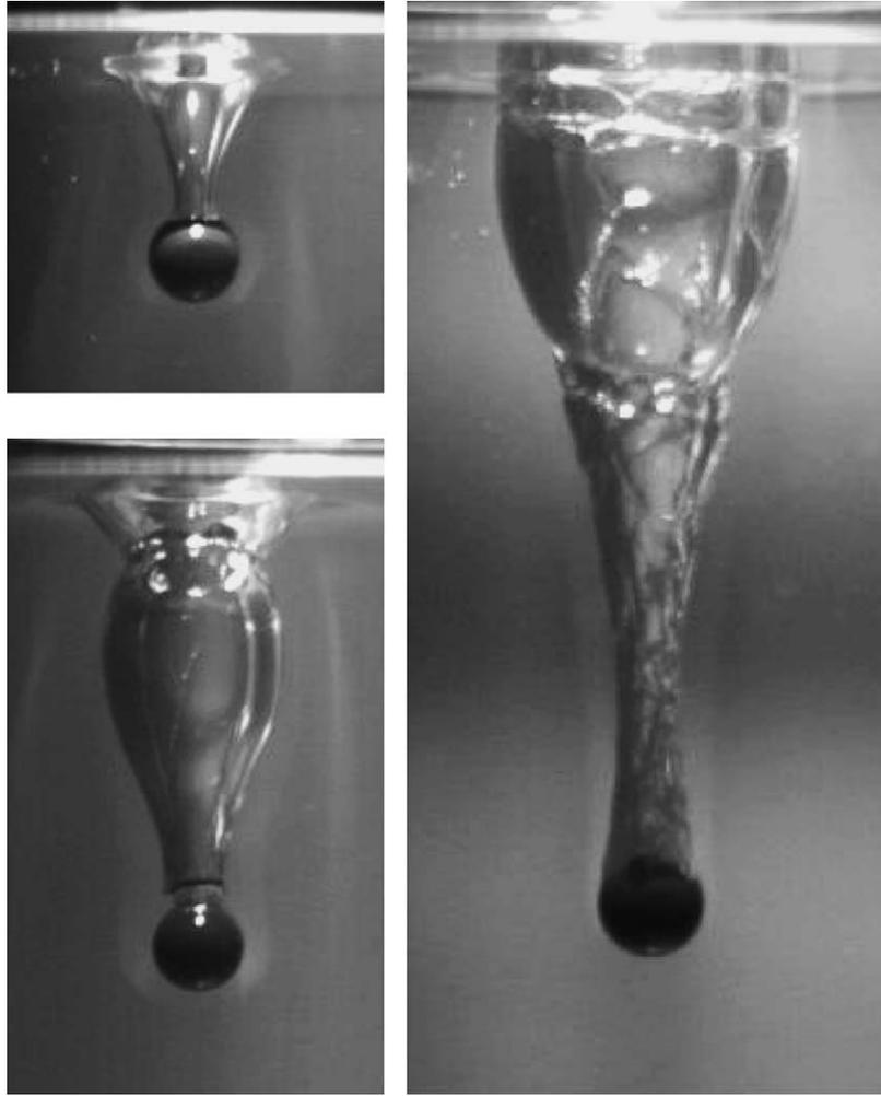
Fig. 8. Different cavity shapes produced by the impact of a  $d = 0.95$  cm silicone nitride sphere on the free-surface of a wormlike micellar fluid ( $\Omega = 9.3$ ) for: (a)  $h_0 = 10$  cm,  $De \simeq 300$ ,  $Fe \simeq 200$ ; (b)  $h_0 = 50$  cm,  $De \simeq 660$ ,  $Fe \simeq 1000$ ; (c)  $h_0 = 127$  cm,  $De \simeq 1050$ ,  $Fe \simeq 2500$ .
